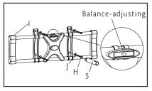
Using balance-adjusting system on the plate, make sure whether wall plate is installed balance. If not, then slide the wall plate let pointer level in the center position.
